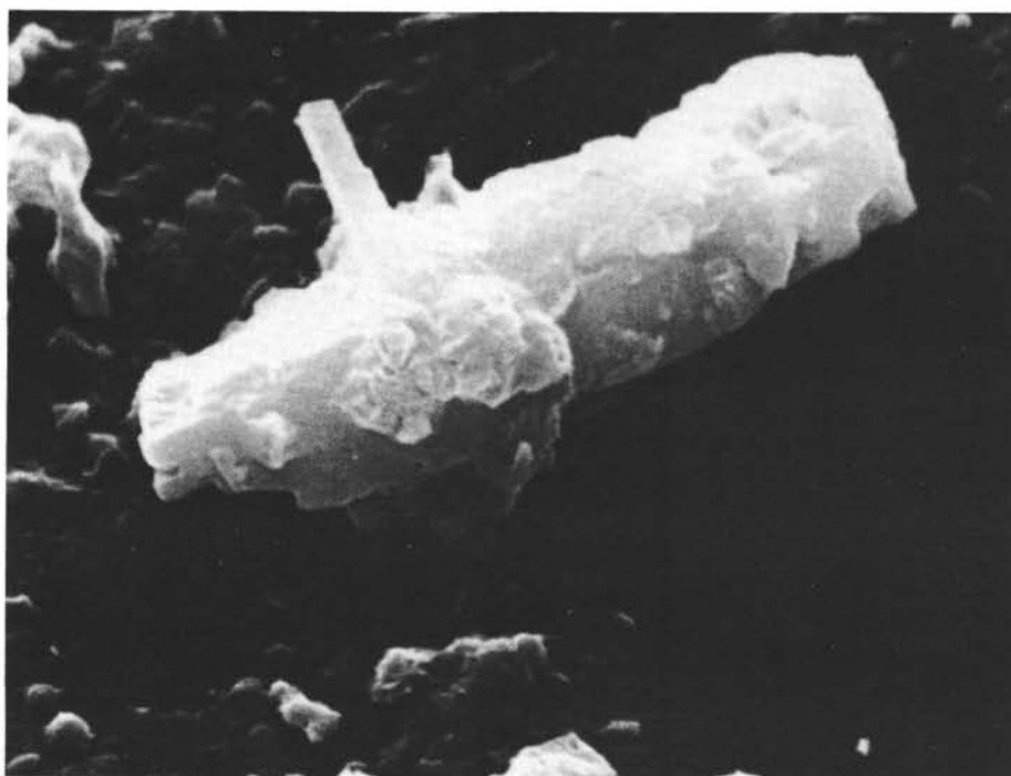
Figure 5. SEM photograph of clinoptilolite from Site 256 (X5000).
